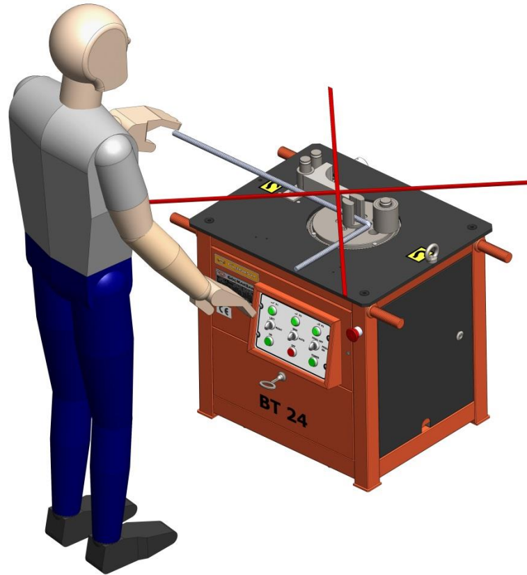
Figure7- Wrong positioning of the person making bend
